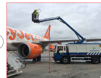
POSITION B- STOP SHORT! OF OUTBOARD ENGINE COWLING. CAGE TO BE ELEVATED ABOVE WINDOW LINE DO NOT SLEW OVER ENGINE PYLON/COWLING
