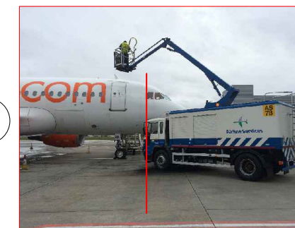
POSITION A- STOP! WHEN MOST FORWARD CORNER OF CAB IS LEVEL WITH SIDE FLIGHT DECK WINDOW. DO NOT DRIVE PAST THIS POINT. CAGE MUST BE ELEVATED ABOVE THE HEIGHT OF THE FUSELAGE
