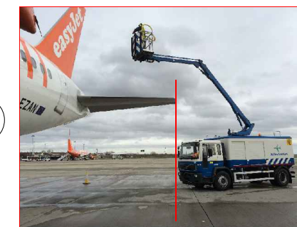
POSITION D- STOP! BEFORE OR WHEN MOST FORWARD CORNER OF CAB IS LEVEL WITH TIP OF HORIZONTAL STABILISER. DO NOT DRIVE RIG FORWARD OF THIS POINT. CAGE MUST BE ELEVATED ABOVE THE WINDOW LINE TO STAY CLEAR OF ENGINE EXHAUST
