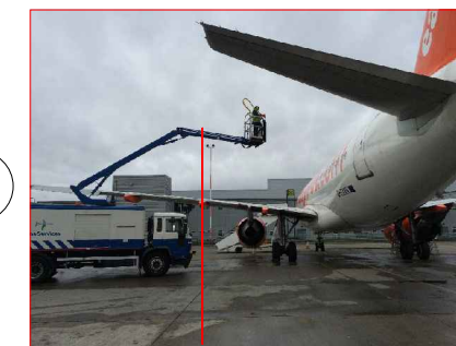
POSITION C- STOP! BEFORE FRONT OF CAB IS LEVEL WITH FAIRING OUTBOARD OF ENGINE. DO NOT DRIVE PAST THIS POINT. CAGE MUST BE ELEVATED ABOVE THE WINDOW LINE TO STAY CLEAR OF THE ENGINE EXHAUST
