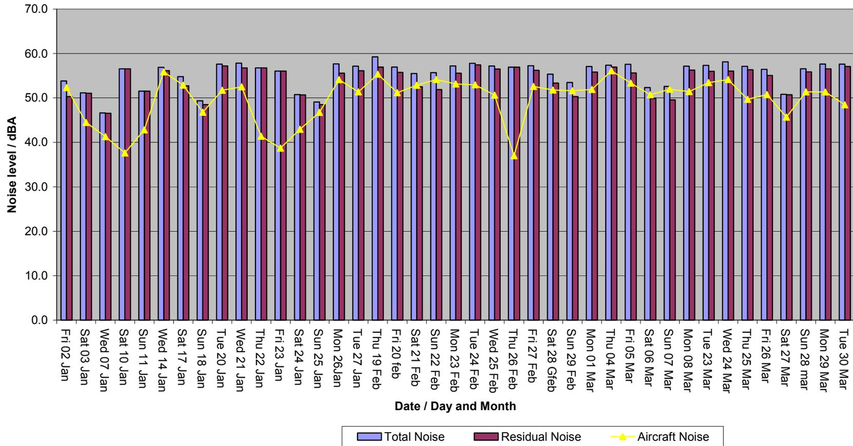
**Figure 10: Contribution of Aircraft Noise and Residual Noise to average daily Total Noise level (LAeq value) for days on which Aircraft Noise events at Harlow in January to April 2008**
