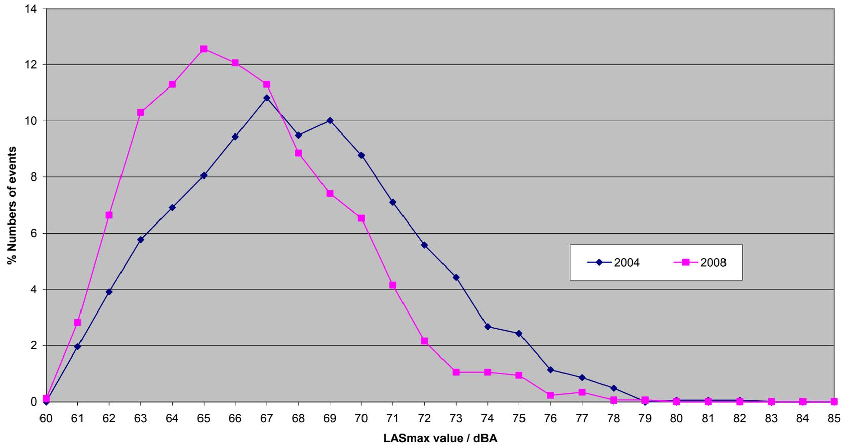
Figure 7: Cumulative statistical analysis of maximum levels of aircraft noise events (LASmax values) at Harlow during survey periods in 2004 and 2008
