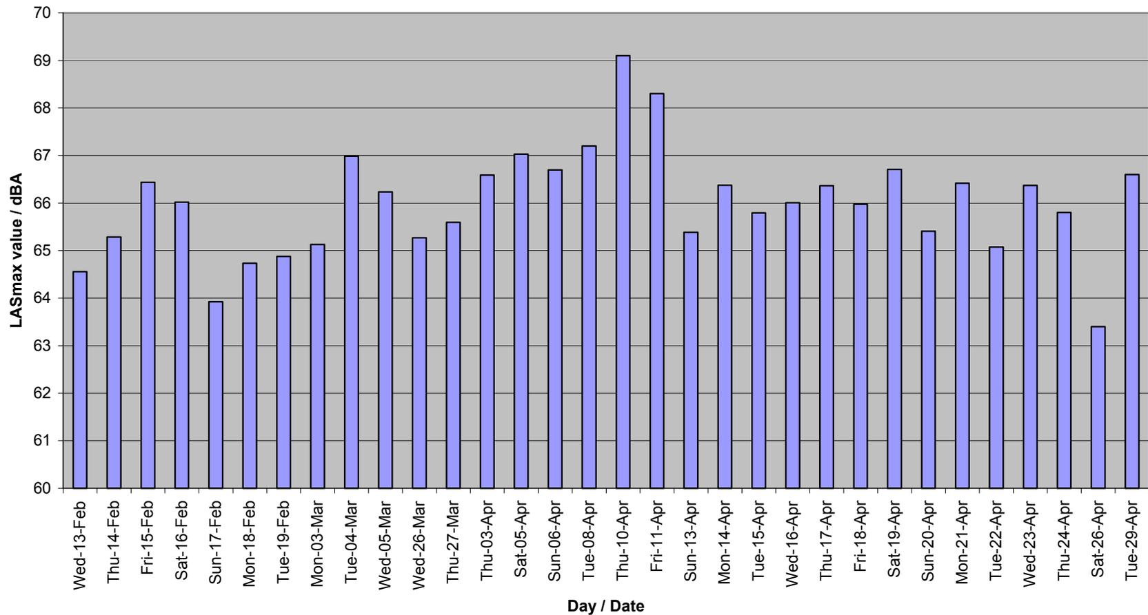
**Figure 6: Statistical analyses of maximum levels of aircraft noise events (LASmax values) at Harlow during survey periods in 2004 and 2008**
