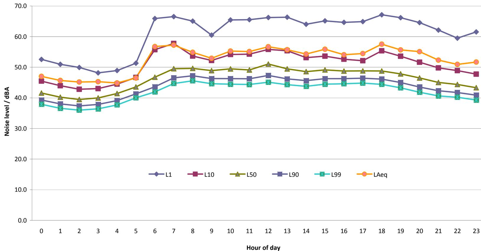
**Figure 7: Noise Climate at Hatfield Heath Essex during October, November and December 2009 showing average values for each hour of day of total noise, aircraft noise and residual noise (LAeq values)**
